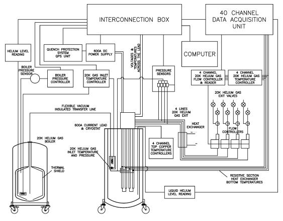
Fig. 1. Schematic of the test-bed including 20 K helium gas generator, test cryostat, instrumentation, and control circuits for temperature and gas flow.
