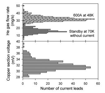
Fig. 4. Distribution histograms of steady state 20 K gas flow rate at full current and standby (upper pane) and voltage drop along the resistive section at 600 A (lower pane).
