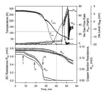
Fig. 2. Cool down time series of 20 K gas flow rate, resistive-HTS junction temperature  $T_{HEX}$ , 20 K inlet temperature  $T_{He}$ , and liquid helium level  $H_{He}$  in the upper pane and resistance of the resistive copper section  $R_{Cu}$  and HTS section  $R_{SC}$  in the lower pane.
