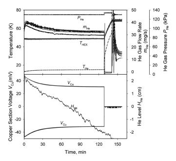
Fig. 3. Full current and standby time series of 20 K gas flow rate, resistive-HTS junction temperature  $T_{HEX}$ , 20 K inlet temperature  $T_{He}$  and pressure  $p_{He}$  in the upper pane and voltage drop  $V_{Cu}$  along the resistive copper section and liquid helium level  $H_{He}$  in the lower pane.
