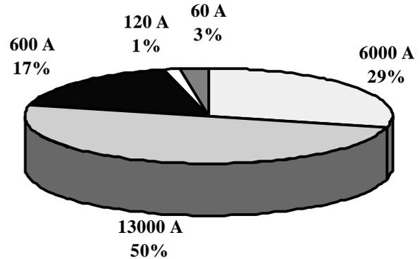
Fig. 1. Current ratings of the LHC current leads.
