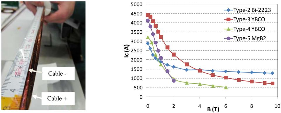
Fig. 1. (a) Twisted-pair cable; (b)  $I_c$  ( $1 \mu\text{V}/\text{cm}$  criterion) measured on one cable of the twisted-pair assembly at 4.2 K and in field. The field is oriented perpendicular to the flat plate supporting the twisted pair cable.
