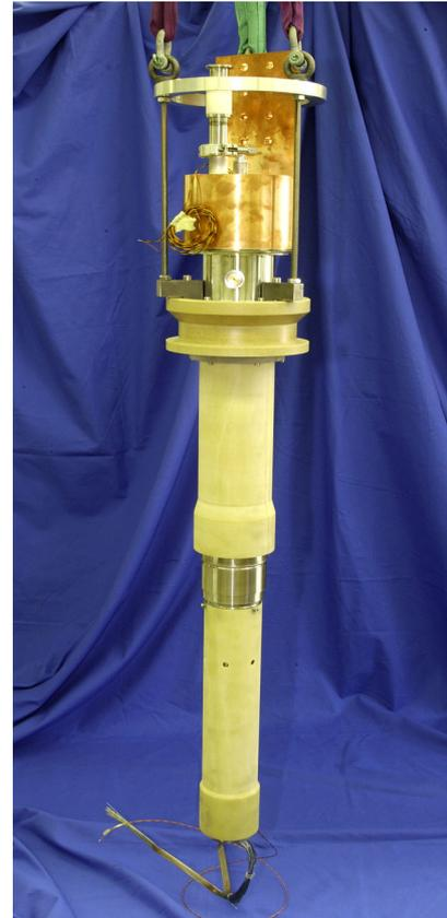
**Figure 1.** 13000 A lead schematic and prototype
