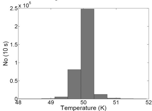
Figure 2: Histogram of the temperatures at  $T_{HTS}$  for all 122 HTS leads during the 8 hour run in sector 5-6.
