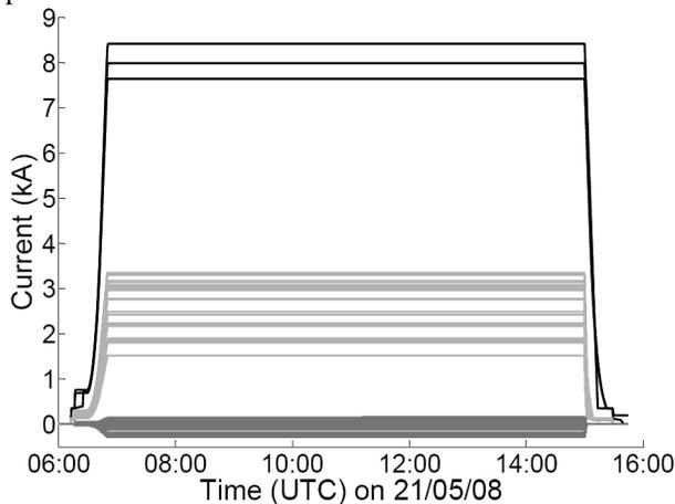
Figure 3: The currents during the eight hour run, including the powering up/down transients. The 13 kA circuits are shown in black, 6 kA in light grey, and 600 A in dark grey.
