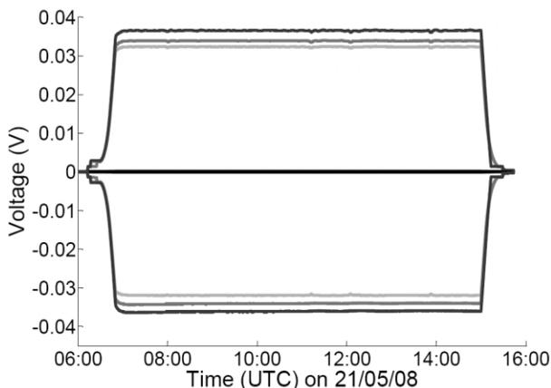
Figure 4: The voltages for the 13 kA circuits during the 8 hour run, including the powering up/down transients. HTS voltages are shown in black, resistive section voltages for the leads transporting 8.42 kA in dark grey, 7.99 kA in lighter grey, and 7.64 kA in lightest grey.
