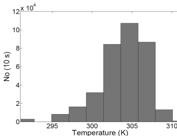
Figure 1: Histogram of the temperatures at  $T_{WARM}$  for all 122 HTS leads during the 8 hour run in sector 5-6.
