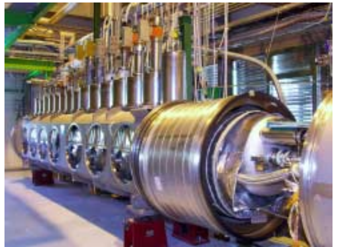
Fig. 4. Prototype HTS leads integrated in the String 2.
