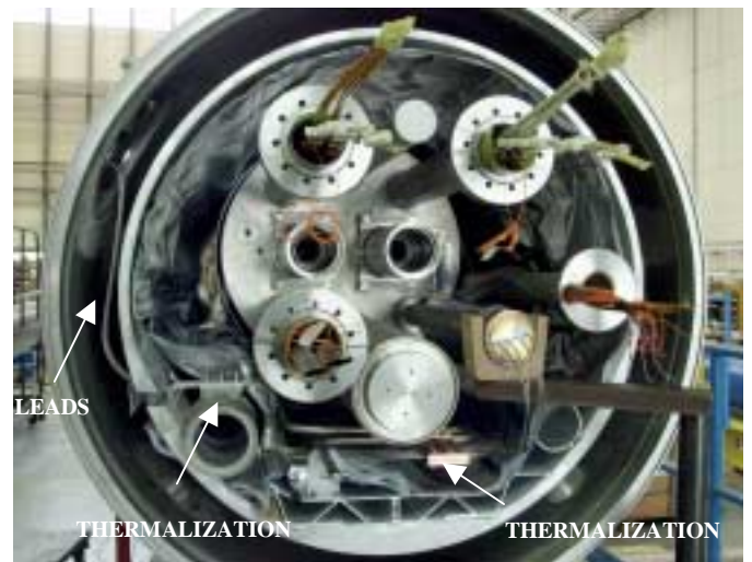
Fig. 5. Prototype 60 A leads integrated in SSS3.
