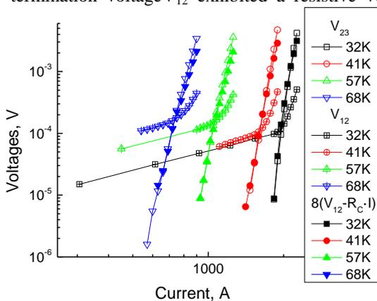
Fig. 4. V-I characteristics of a terminal ( $V_{12}$ ) and the complete strand ( $V_{23}$ ) for Type-2 at different temperatures.
