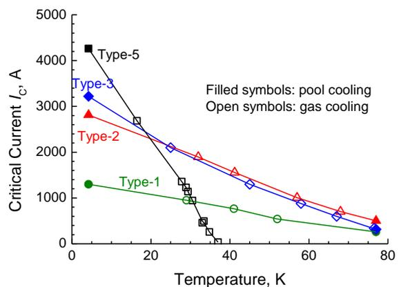
Fig. 5. Critical current  $I_C$  as a function of temperatures for different cable types.
