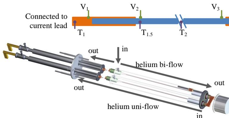
Fig. 1. An illustration of the cryostat for the electric tests of twisted-pair HTS cables. The uni- and bi-flow configurations for the cooling helium gas and the layout of the instrumentations are shown as indicated.
