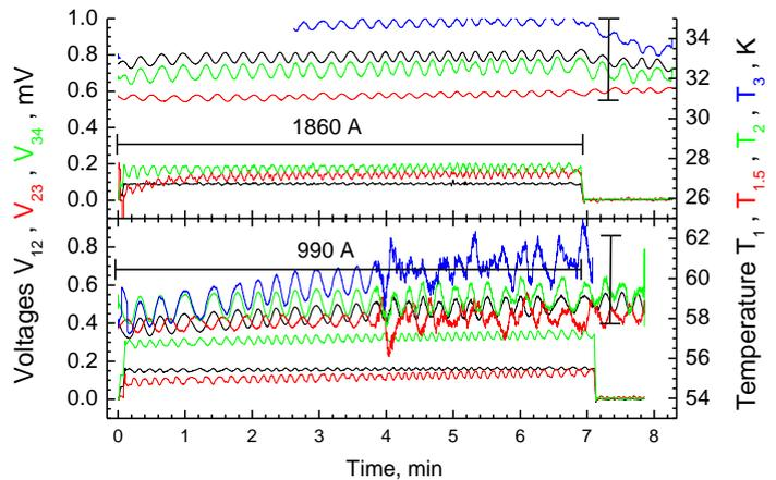
Fig. 6. Time series of voltage and temperature for Type-2 cable at near critical currents at  $32 \text{ K}$  and  $67 \text{ K}$ , showing stability for over 5 minutes.
