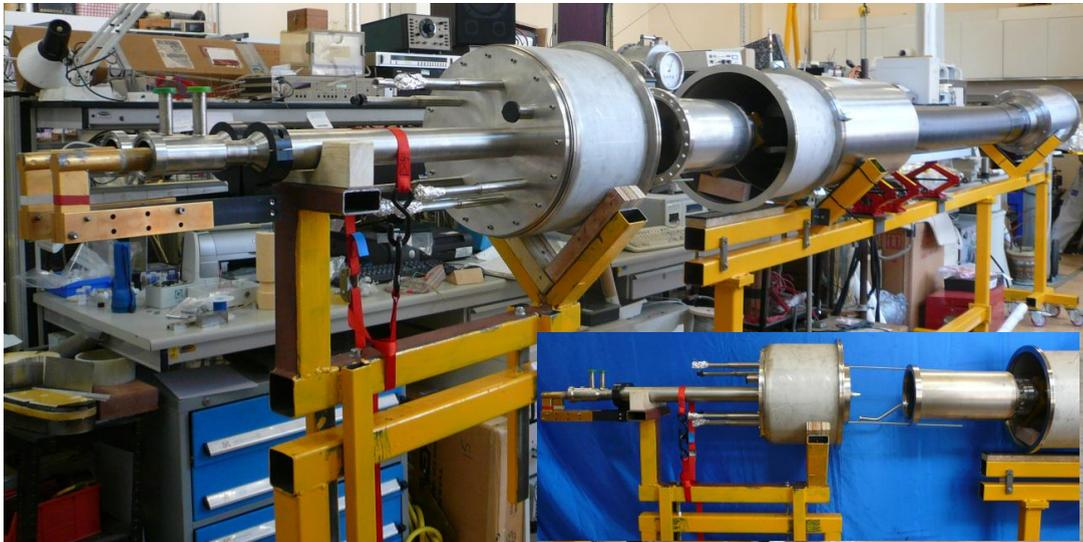
Fig. 2. A 5 m semi-flexible cryostat commissioned at University of Southampton for the test of HTS links. The inset shows the interface between the cable vessel and the current-lead unit.
