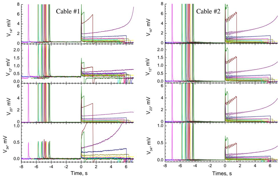
Fig. 3. Voltage traces along two strands of Type-3 cables at 50 K in a uni-flow configuration upon the injection of current pulses. Each colour corresponds to a current value ranging from 880 A to 1100 A in 20A intervals. Thermal runaway occurred at 1160 A.
